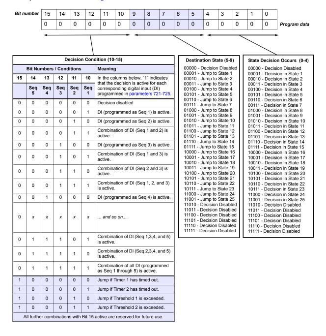
Figure 7-3: Seq Decision Parameter's Bit-Packed Definition
