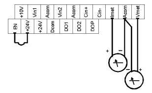
Figure 4-8: Connections for Process Meters
