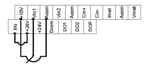
Figure 4-6: Connections for Speed Potentiometer
