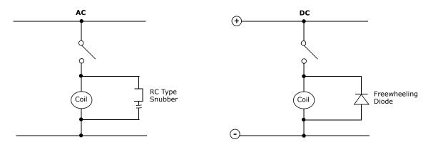
Figure 4-10: Connection Diagram for AC and DC Relay Coils and Solenoids
