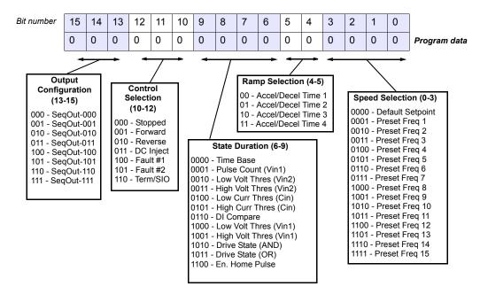
Figure 7-1: Seq Cntl Parameter, Bit Definition
