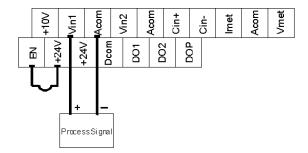
Figure 4-7: Connections for Process Signal
