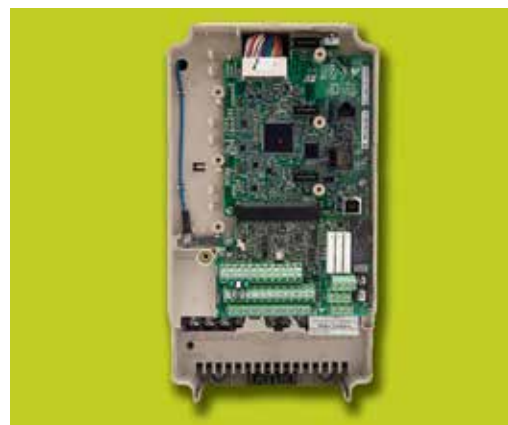
Easy Power & Control Terminal Access
