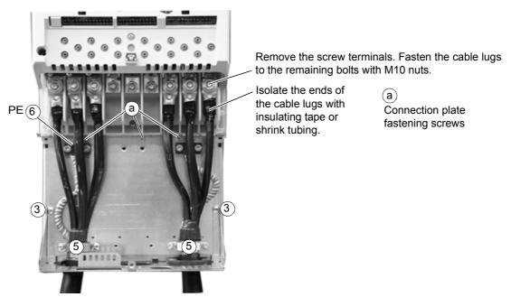
Frame size R6: Cable lug installation [16 to 70 mm<sup>2</sup> (6 to 2/0 AWG) cables]
