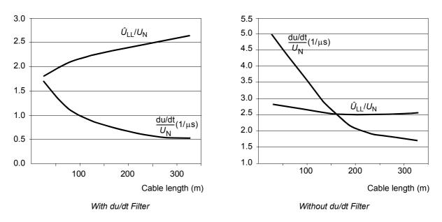
**Note 9:** Sine filters protect the motor insulation system. Therefore, du/dt filter can be replaced with a sine filter. The peak phase-to-phase voltage with the sine filter is approximately 1.5 ×  $U_{\rm N}$ .
