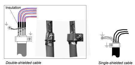
When the outer surface of the shield is covered with non-conductive material:
