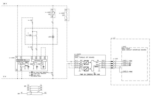
Safe torque off circuit diagram
