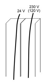
Lead 24 V and 230 V (120 V) control cables in separate ducts inside the cabinet.
