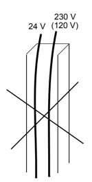
Not allowed unless the 24 V cable is insulated for 230 V (120 V) or insulated with an insulation sleeving for 230 V (120 V).
