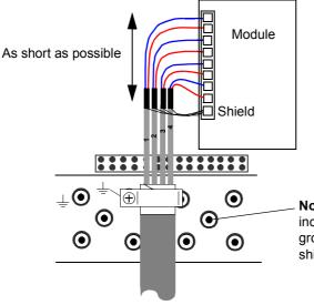
**Note:** The RDIO module does not include a terminal for cable shield grounding. Ground the pair cable shields here.
