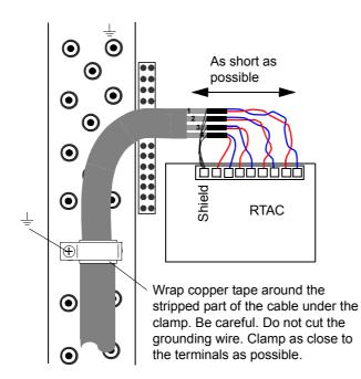
**Note 1:** If the encoder is of unisolated type, ground the encoder cable at the drive end only. If the encoder is galvanically isolated from the motor shaft and the stator frame, ground the encoder cable shield at the drive and the encoder end.
