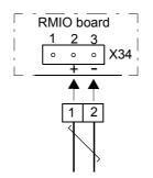
Connection of a two-way connector
