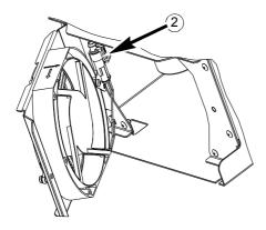
3. Undo the fastening screws of the fan.
