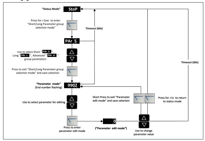
NOTE When attempting to edit a parameter the drive must be stopped (not running), if not "L" will be shown on the left side of the display.
